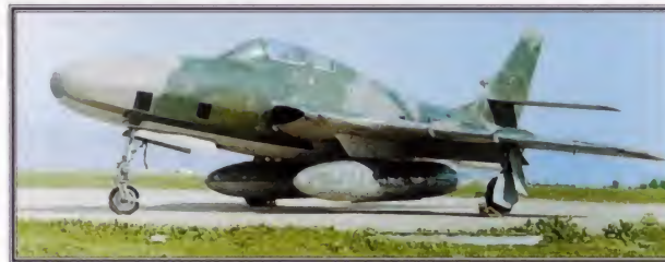
▲ Photo jet The RF-84F was a photo reconnaissance variant, with side-mounted intakes to allow for the large camera-filled nose section.
